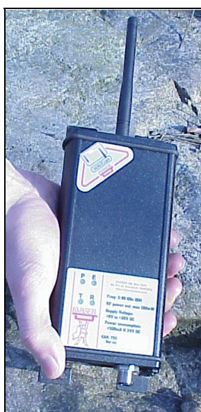
Fig. 5: WaveCAN unit for testing and evaluation of Bluetooth/CAN properties
